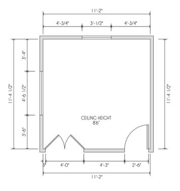
4 Measure the overall widths and lengths of the room. This is very important as it will help double-check the incremental measurements.
